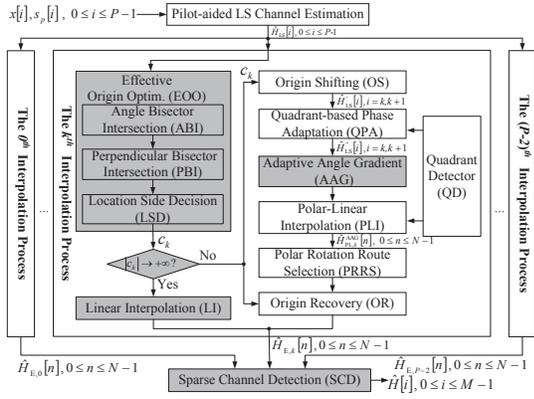
Fig. 1. The system framework of E-APLI-CE.
